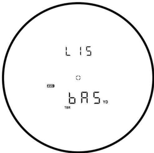
**Internal display as seen through the RX-1400i TBR/W after the power button is pressed** - Allows you to confirm the output settings or load that is actively selected in the rangefinder.
