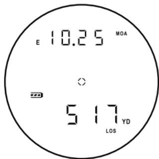
TRIG, a function that is included to support tradesmen and sportsmen alike, displays the true horizontal range and true vertical range, which is based upon trigonometry using angle
