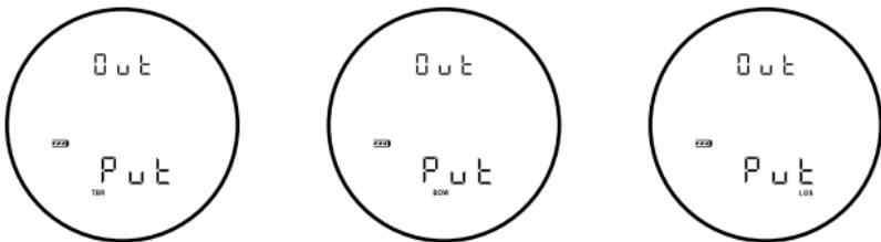
To activate TBR, BOW, or LOS mode, press the POWER button, then press the MODE button for <1 second and release to enter the menu. While “Out Put” is shown in the display, press and release the POWER button to rotate through TBR, BOW, and LOS modes. Once the desired mode is displayed, press the MODE button.
