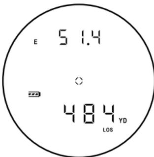
MIL will display the appropriate amount of holdover in milliradians to use, which is based upon the ballistics group and sight-in distance you will choose in a later mode. The lower display shows the line of sight distance to the target. The upper display shows the appropriate number of mils to hold over or
