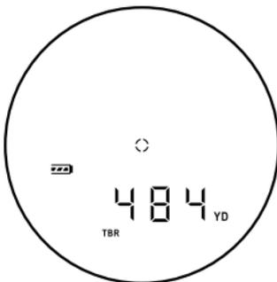
This is the range you will want to use when shooting, rather than the line of sight distance, which may contain gross errors depending upon the shot angle. Readings will be displayed with equivalent horizontal range in the lower portion of the display.
