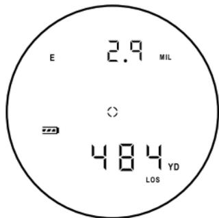
MOA will show the minute-of-angle adjustment for your target, which is based upon the ballistics group and sight-in distance you will choose in a later mode.
